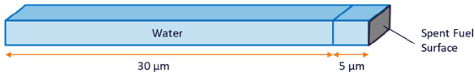
Figure 1: Sketch of the system considered in the preliminary calculations. The model considers two domains: a 30\ \mu\text{m} domain of water and a 5\ \mu\text{m} domain of water in contact with the spent fuel surface. The water domain considers aqueous speciation only, while the second domain also considers reactions with the solid surface.
