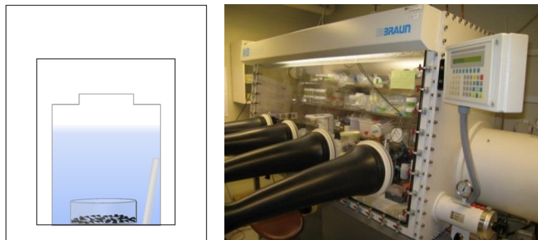
Figure 1: Schematic view of closed plastic vessel ( V = 60 \text{ mL} ) (left) in which the experiments will be conducted in the anaerobic glove box (right). \text{UO}_2 fragments are placed in the zircaloy saucer and the iron strip is leaning on the vessel wall in experimental media.
